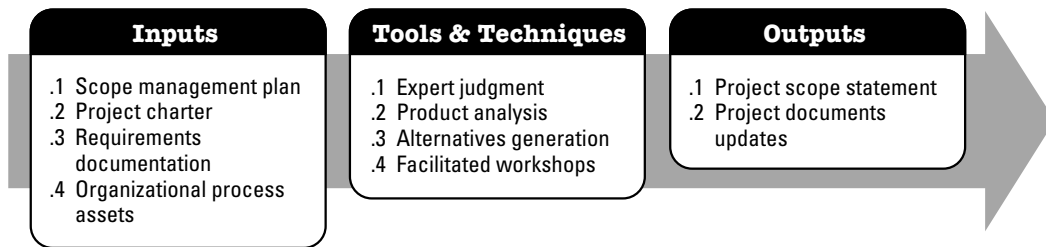
Figure 5-7. Define Scope: Inputs, Tools & Techniques, and Outputs
